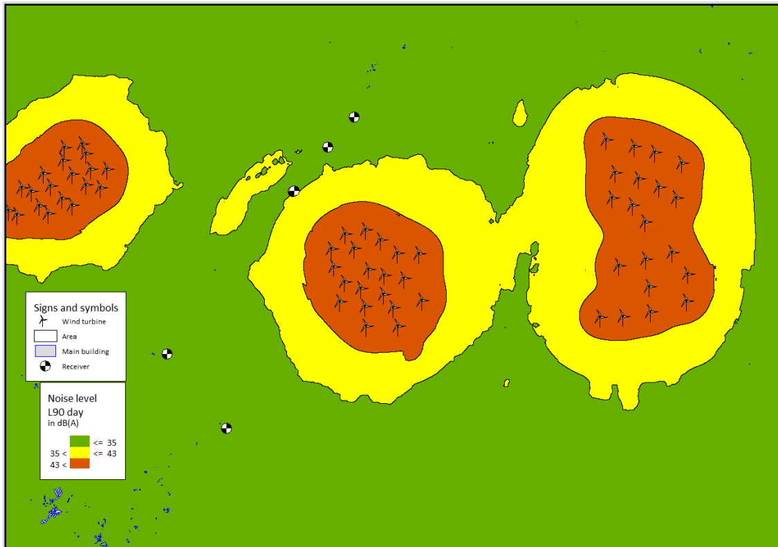
Figure 8.2 Predicted Noise Contours for the Proposed Development and existing wind farms for 10 m/s standardised 10 m height wind speed
