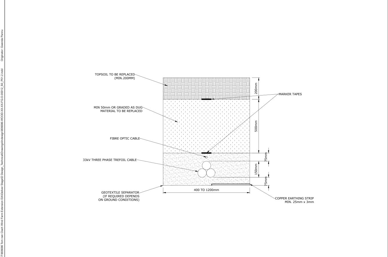
Title: Typical Cable and Trench Cross Section Project: Tom na Clach Wind Farm Extension Source: Client: Infinergy Drawn by: Checked: panng hughg Date: Figure: November 2021 3.11 Revision No: Scale: 1:10 P01.2
