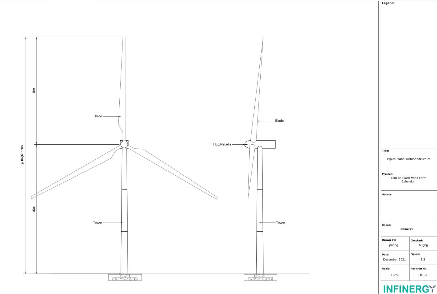
Typical Wind Turbine Structure Project: Tom na Clach Wind Farm Extension Source: Client: Infinergy Drawn by: Figure: December 2021 1:750
