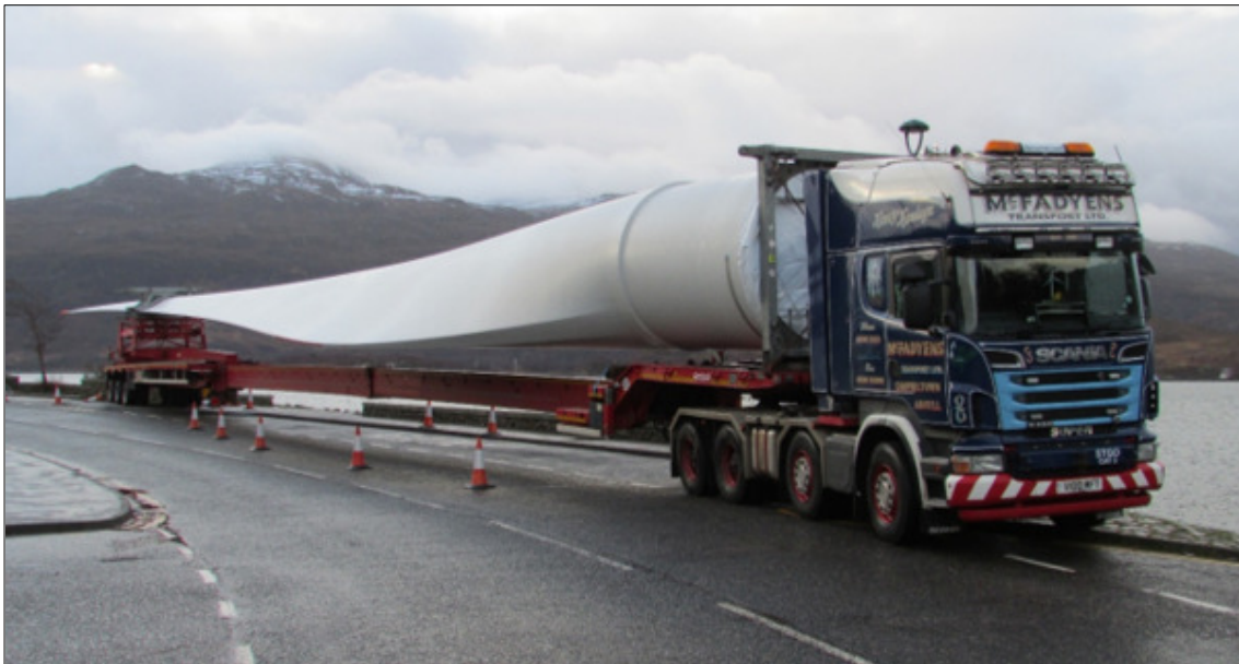
Figure 3 Super Wing Carrier with Loaded Turbine Blade
